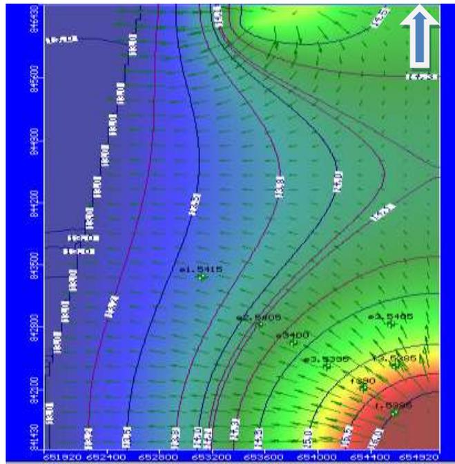
**Figure (7):** Water level contour map of the steady state during year 2005.
