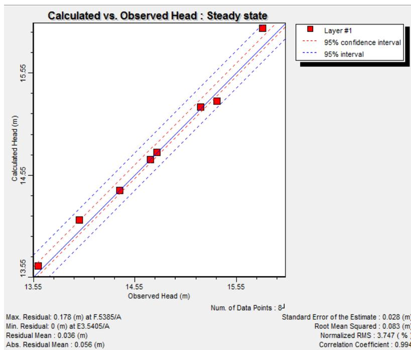
**Figure (8):** Relation between the observed and the calculated head, steady state calibration
