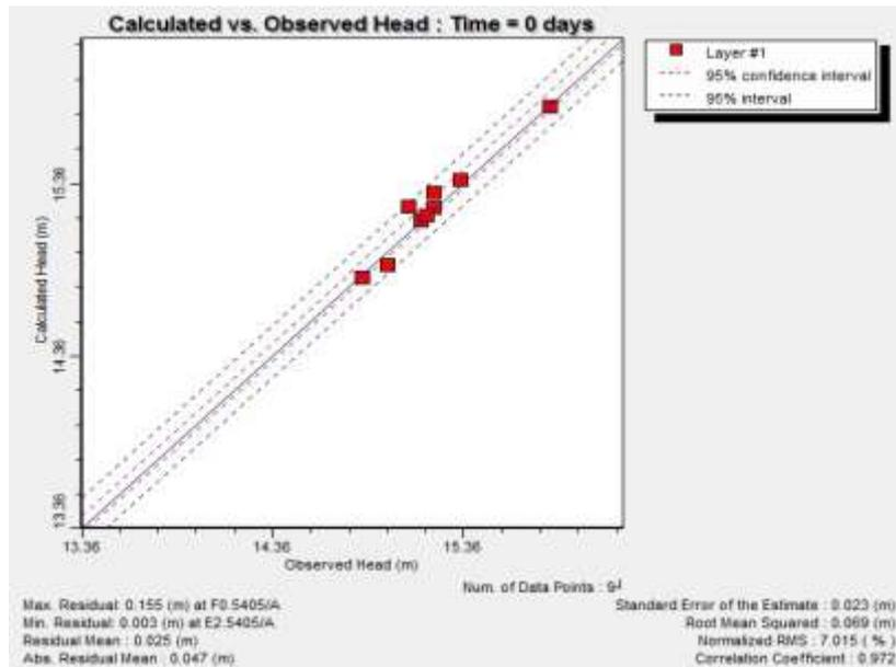
Figure (10): Relation between the observed and the calculated head, unsteady state calibration.
